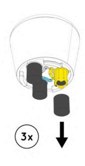
Screw back the protection cap before placing Ico into the water
